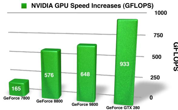
In contrast, NVIDIA GPU performance went from 165 GFLOPS in the GeForce 7800 series GPU's to 933 GFLOPS in the GTX 280 GPU series.
