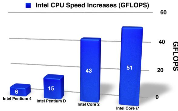
The chart to the right shows increases in speed between Intel's Pentium 4 series and the Intel Core i7 series.
